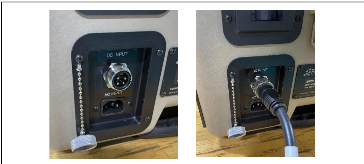
Figure 9: DC Power Connection
